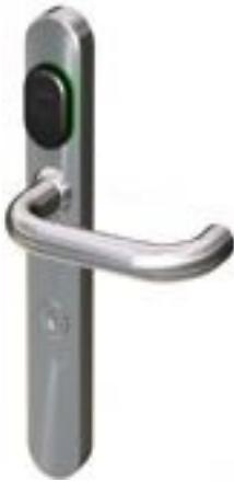
**The Kaba Elolectric C-Lever is a stand alone, mechatronic door fitting whose electronics are integrated within. Access is gained using a choice of contact free media such as keys, ID cards or fobs when fitted with the renowned LEGIC chip. If a valid medium is read by the electronics, a motor engages the handle coupling and the door can be opened for 5 seconds. In addition, the LEGIC chip allows other applications such as time & attendance, cash-free payment and audit trail.**
