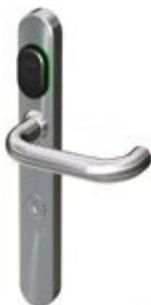
**The Kaba Elolegic C-Lever is a stand alone, mechatronic door fitting whose electronics are integrated within. Access is gained using a choice of contact free media such as keys, ID cards or fobs when fitted with the renowned LEGIC chip. If a valid medium is read by the electronics, a motor engages the handle coupling and the door can be opened for 5 seconds. In addition, the LEGIC chip allows other applications such as time & attendance, cash-free payment and audit trail.**
