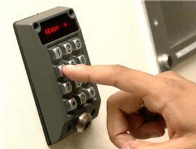
Access control systems (ACS), where deployed, using database-driven identity management and token-based access, allow not just control of access, but also up-to-date and accurate accounting for personnel on site. This greatly aids health and safety. There is an administrative overhead on management of these systems and the requirements for robustness above apply equally to them, but the cost-benefit ratio is usually sufficiently compelling for a larger site to elect deployment.
