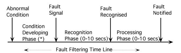
= The time period before an abnormal condition becomes a fault condition (the condition developing phase) will vary e.g. see Table 16
